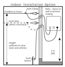
be used, alternatively galvanised pipe or steel posts can be used as earth rods. Earth rods should be driven 2m (6.5ft) into the soil and spaced at least 3m (10ft) apart.
